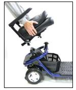
Figure 13. Removing the Seat
