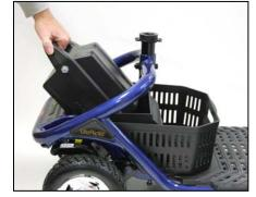
Figure 21. Battery Pack Installation
