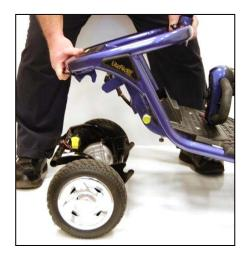
Figure 18. Lifting the Frame
