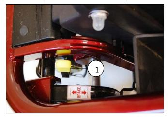
Figure 10. Drive Mode (Brake Engaged)
