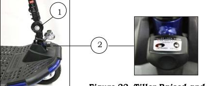
Figure 22. Tiller Raised and Unlocked
