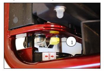
Figure 9. Freewheel Mode (Brake Disengaged)
