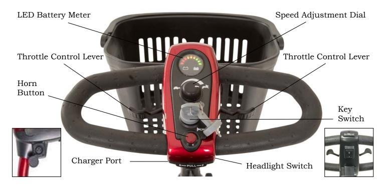
Figure 5. LiteRider<sup>TM</sup> Delta Tiller Control Panel
