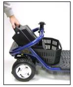
Figure 14. Removing the Battery Pack
