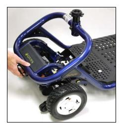
Figure 17. Releasing the Drivetrain
